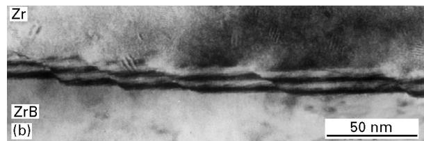
Figure 4 Bright-field TEM image of an \alpha\text{Zr-ZrB} interface exhibiting a curved boundary (a) which can be resolved as facets (b) at higher magnification.
